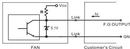
$V_{cc}$ =From + 5 To + 80 VDC ( Generally using + 12 or + 24VDC )
