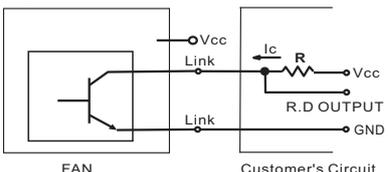
$V_{cc}$ =From + 5 To + 28 VDC ( Generally using + 12 or + 24VDC )
