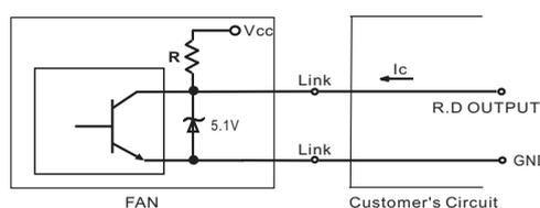
$V_{cc}$ =From + 5 To + 28 VDC ( Generally using + 12 or + 24VDC )
