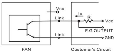
$V_{cc}$ =From + 5 To + 80 VDC ( Generally using + 12 or + 24VDC )
